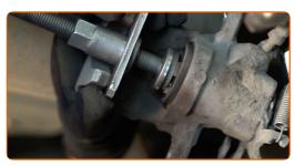
Install the brake caliper and fix it. Use a combination spanner #17. Use a drive socket #14. Use a torque wrench. Tighten it to 35 Nm torque.
