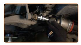
Unscrew the fastener connecting the stabilizer link to the shock strut. Use HEX No.H6. Use a drive socket #17. Use a ratchet wrench.
