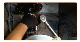
Tighten the fastener connecting the stabilizer link to the stabilizer bar. Use a drive socket #17. Use a torque wrench. Tighten it to 74 Nm torque.
