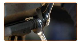
10 Remove the brake caliper.
