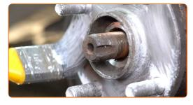
69 Install the brake disc.
