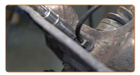
Tighten the lower fasteners connecting the shock strut to the steering knuckle. Use a combination spanner #19. Use a drive socket #19. Use a torque wrench. Tighten it to 164 Nm torque.
