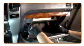
Remove the cabin air filter housing.
