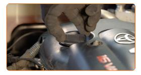
Run the engine for a few minutes. After the oil pressure warning light goes out, stop the engine.
