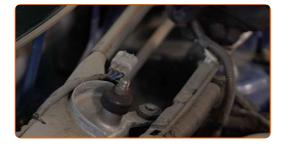
Unscrew the fasteners of the windscreen wiper linkage panel. Use a drive socket #10. Use a ratchet wrench.
