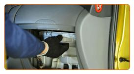
4 Remove the filter element from the filter housing.
