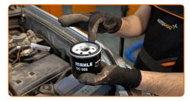
Screw the new filter into its place. Use the 76-14F socket. Use a torque wrench. Tighten it to 20 Nm torque.
