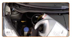
Replacement: engine oil and filter – TOYOTA MR2 III Convertible (W30).
