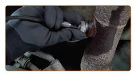
Tighten the oxygen sensor fastener. Use a combination spanner #22. Use a torque wrench. Tighten it to 41 Nm torque.
