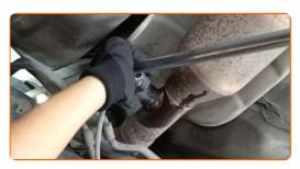
Clean the oxygen sensor mounting seat. Use WD-40 spray.
