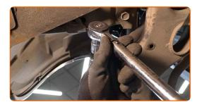
Tighten the fastener connecting the stabilizer link to the shock strut. Use a drive socket #17. Use a torque wrench. Tighten it to 74 Nm torque.
