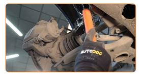
Unscrew the fastener connecting the stabilizer link to the stabilizer bar. Use a drive socket #17. Use a tap wrench.
