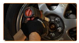
Lower the car and working in a cross order, tighten the wheel bolts. Use wheel impact socket #21. Use a torque wrench. Tighten it to 103 nm torque.
