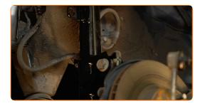
Replacement: anti roll bar links – TOYOTA Matrix I MPV (E130). Tip from AUTODOC experts:
