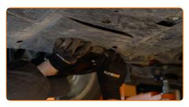
Tighten the fasteners of the oil pan lower cover.
