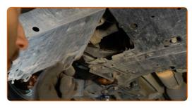
Put a waste oil container with at least 5 l capacity under the drainage hole.
