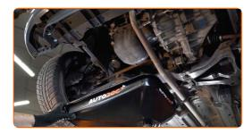
9 Unscrew the oil filter. Use the 76/14-F socket.
