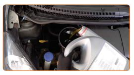
Replacement: engine oil and filter – TOYOTA Liteace Minibus (M30).
