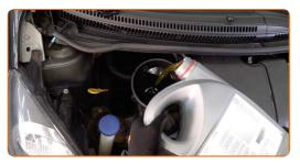
Replacement: engine oil and filter – TOYOTA Liteace Minibus (M20).
