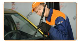
Remove the blade from the wiper arm.
