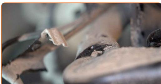
**16** Unscrew the fastener connecting the trailing arm to the car body. Use a combination spanner #19.
