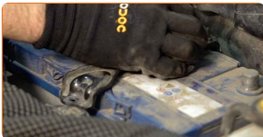
**44** Screw in the battery hold down clamp. Use a drive socket #10. Use a ratchet wrench.
