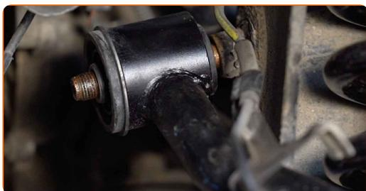
**26** Attach the upper control arm to the steering knuckle.
