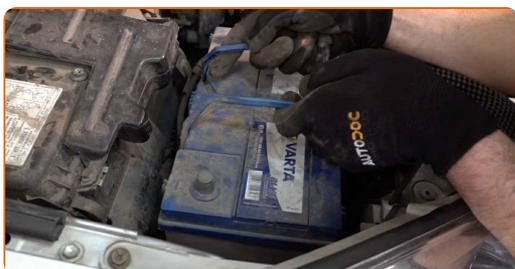
**43** Install the battery hold down clamp.
