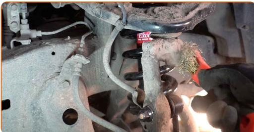
**14** Unscrew the ABS cable holder. Use a drive socket #12. Use a ratchet wrench.
