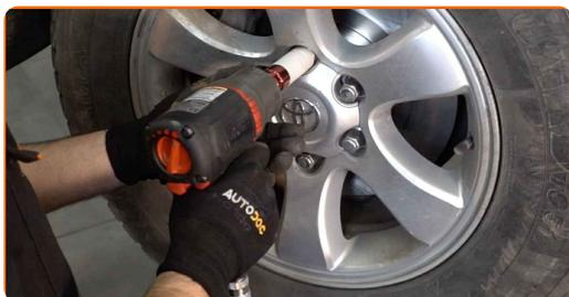
**41** Lower the car and working in a cross order, tighten the wheel bolts. Use a torque wrench. Tighten it to 112 nm torque.
