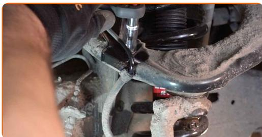
**15** Remove the mounting bracket of the ABS sensor wiring from the upper arm.
