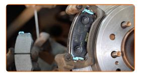
Replacement: brake pads – TOYOTA LAND CRUISER Pickup (\_J7\_). Tip from AUTODOC experts:
