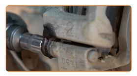
10 Remove the brake caliper.
