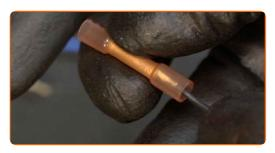
16 Crimp the solder sleeves. Use crimping pliers.
