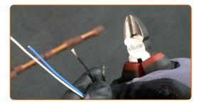
Place the heat shrink tubing on the oxygen sensor wiring.
