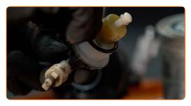
Screw in the water-in-fuel sensor.
