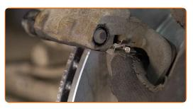
Treat the brake caliper piston. Use a wire brush. Use a brake cleaner.
