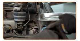
8 Unscrew the bracket of the water-in-fuel sensor. Use a drive socket #8.
