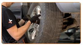
Replacement: brake pads – TOYOTA LAND CRUISER 150 (KDJ15\_, GRJ15\_).
