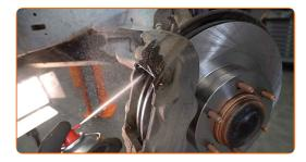
Replacement: brake pads – TOYOTA LAND CRUISER 150 (KDJ15\_, GRJ15\_). Tip:
