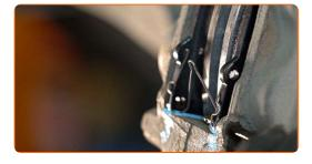
Install the brake pads retaining clips.
