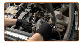
Tighten the fuel filter fasteners. Use a drive socket #12. Use a ratchet wrench.
