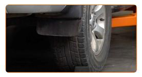
Loosen the wheel mounting bolts. Use wheel impact socket #21.
