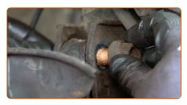
Install the steering knuckle on the CV axle.
