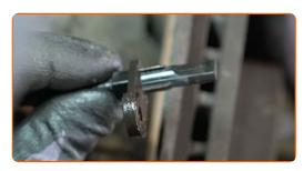
Unscrew the fastener connecting the drive shaft to the wheel hub. Use 12-point socket No.30. Use a ratchet wrench.
