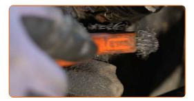
Remove the cotter pin that secures the fastener connecting the ball joint to the steering knuckle. Use a crowbar.
