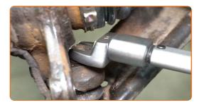
Install the cotter pin that secures the fastener connecting the ball joint to the steering knuckle.
