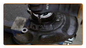
Install the wheel hub on the steering knuckle. Use a bush and bearing driver set.
