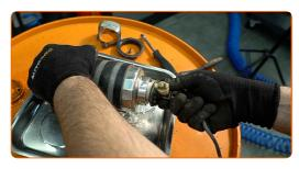
Wait until the fuel is completely drained from the fuel filter.
