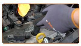
Replacement: spark plugs – TOYOTA Hilux Platform / Chassis (LN\_, \_N1\_).
