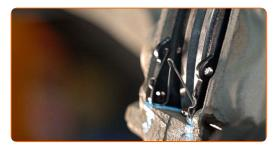
Install the brake pads retaining clips.
