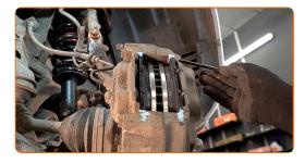
17 Install the retaining spring of the brake pads.
