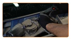
Screw in the fasteners of the fuse box. Use a drive socket #10. Use a ratchet wrench.
