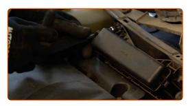
Remove the panel assembled with the windscreen wiper linkage.
