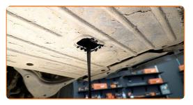
Replacement: engine oil and filter – TOYOTA HIACE IV Box (TRH2\_, KDH2\_). Tip:
