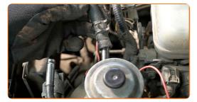
Tighten the fastening clamps of the fuel filter pipes. Use round-nose pliers.
