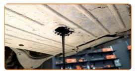
Replacement: engine oil and filter – TOYOTA Hiace / Commuter Minibus V (TRH2\_, KDH2\_). Tip:
