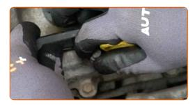
Tighten the fasteners of the wiring harness bracket. Use a drive socket #10. Use a torque wrench. Tighten it to 9 Nm torque.
