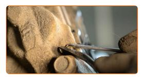
Remove the retainer of the brake pads. Use a pin punch. Use a rubber mallet.
