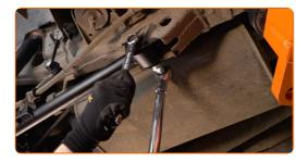
Install the bracket attaching the parking brake cable to the trailing arm. Use a drive socket #12.
