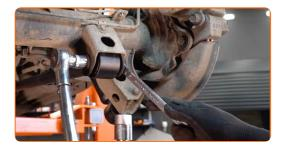
Tighten the fastener connecting the control arm to the car body. Use a combination spanner #19. Use a drive socket #19. Use a torque wrench. Tighten it to 130 Nm torque.
