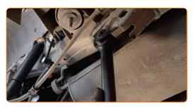
Replacement: rear suspension lower trailing arm – TOYOTA FJ Cruiser (GSJ1\_). Tip from AUTODOC experts:
