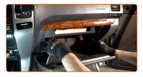
Remove the cabin air filter housing.
