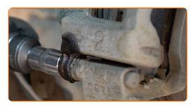
10 Remove the brake caliper.
