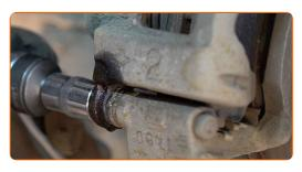
10 Remove the brake caliper.
