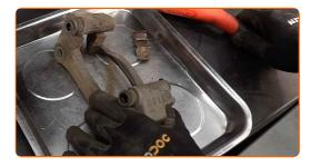
21 Install the brake caliper bracket.
