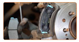
Install the brake caliper and fix it. Use a drive socket #17. Use a torque wrench. Tighten it to 88 Nm torque.
