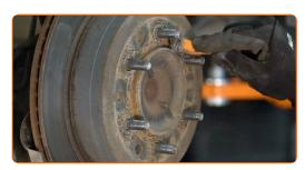
Remove the brake disc. Use a crowbar. Use a rubber mallet.
