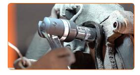
14 Remove the caliper bracket.
