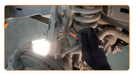
Unscrew the fasteners connecting the stabiliser link to the stabiliser bar. Use a combination spanner #17. Use HEX No.H6.
