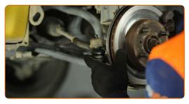
Tighten the fastening nut connecting the tie rod end to the steering knuckle. Use a drive socket #19. Use a torque wrench. Tighten it to 49 nm torque.
