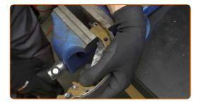
Remove the brake shoe hold-down cup.
