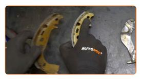
Install the brake shoe adjuster lever.
