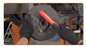
Remove the cap of the parking brake cable fastener.
