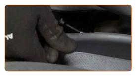
Reinstall the cap of the parking brake cable fastener.
