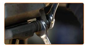
10 Remove the brake caliper.
