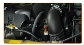
Fasten the clamp on the air intake hose. Use a Phillips screwdriver.
