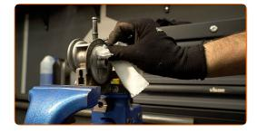
Screw in the new cartridge. Use an oil filter wrench. Use a torque wrench. Tighten it to 14 Nm torque.
