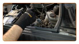
Attach the connector of the water-in-fuel sensor.
