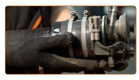
Tighten the clamps of the fuel filter protective case. Use a drive socket #8.
